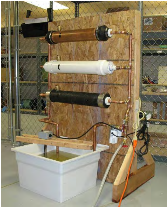
Figure 4. Piping assembly used for laboratory testing. The system consists of a heated water reservoir, a system of pipes, and an electric pump to force the heated water through the pipes. The system was run for two hours prior to testing to ensure that a steady-state pipe temperature had been attained.
