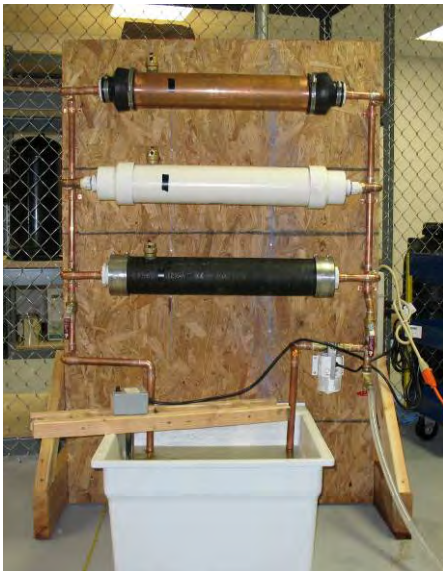
Figure 6. View of the testing equipment as seen from a 10-foot distance, along with the corresponding IR image. Note that all three pipes maintained a temperature of approximately 120° F via the floor-mounted water source. The three pipes appear to have different temperatures based on the thermal image.
